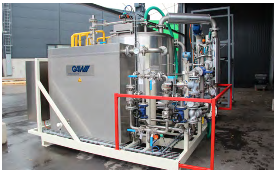
Figure 2. Mobile rental unit GAW starch preparation
