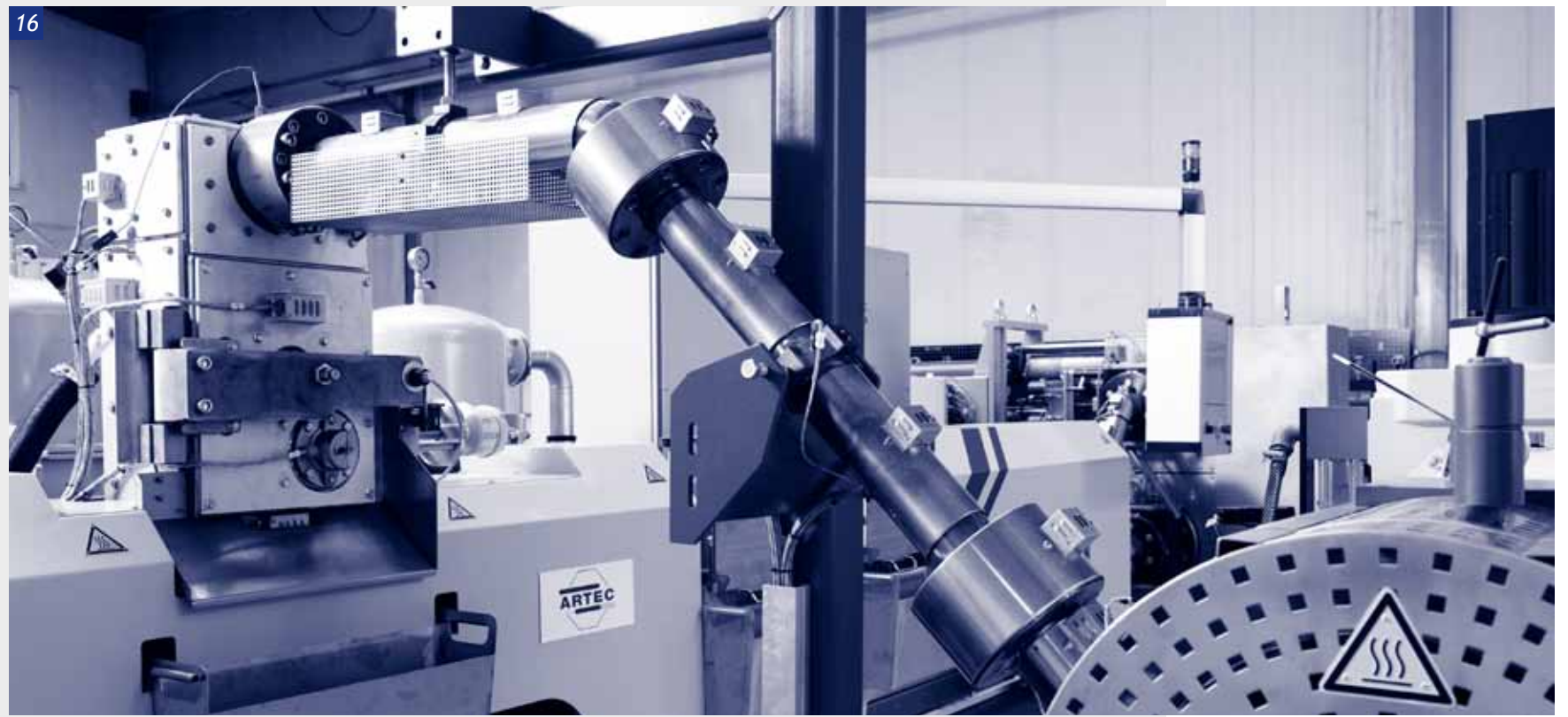
16 The molten material line flows into the vacuum chamber onto a perforated plate where the melt flow is split into four hundred single strands.
