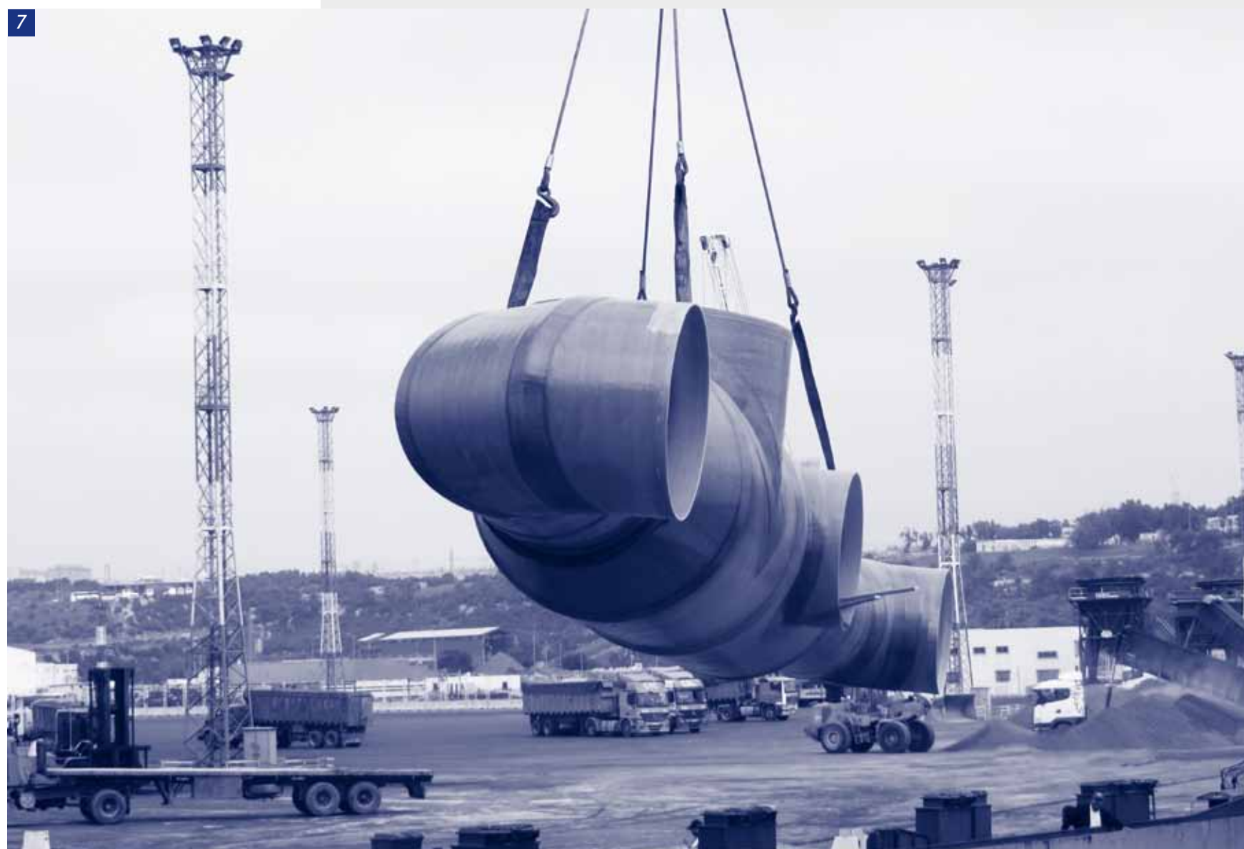
7 Glass fibre reinforced plastic pipework
