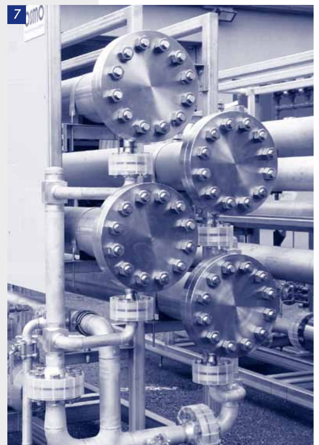
7 Ultra high pressure reverse osmosis system
